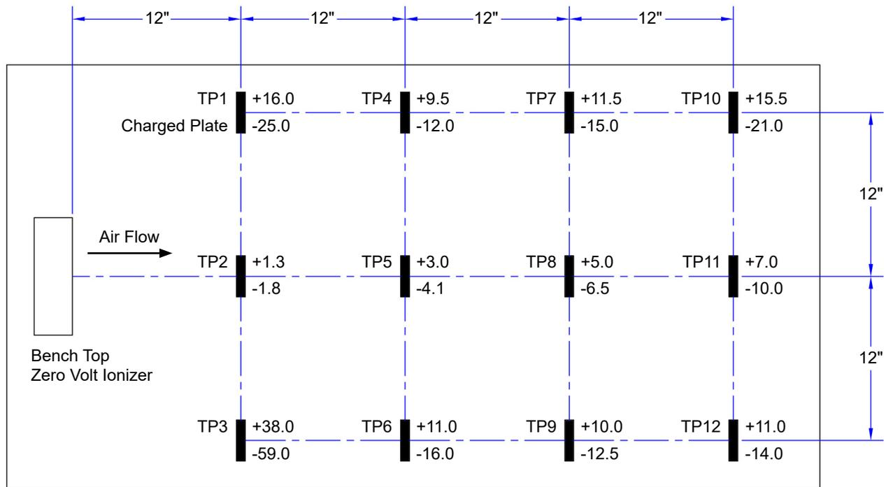
Figure 7. Neutralization (Discharge) Times at 100VAC, 50Hz input
