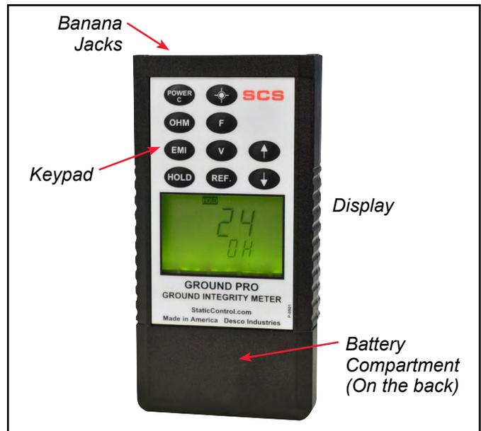
Figure 2. Ground Pro Meter features and components
