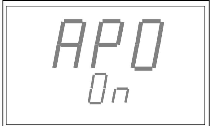
Figure 4. Automatic Power Off (APO) display
