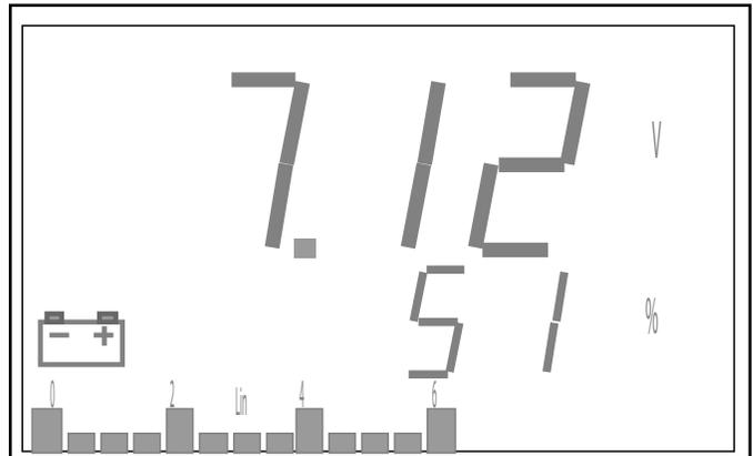
Figure 5. Battery voltage and percentage.
