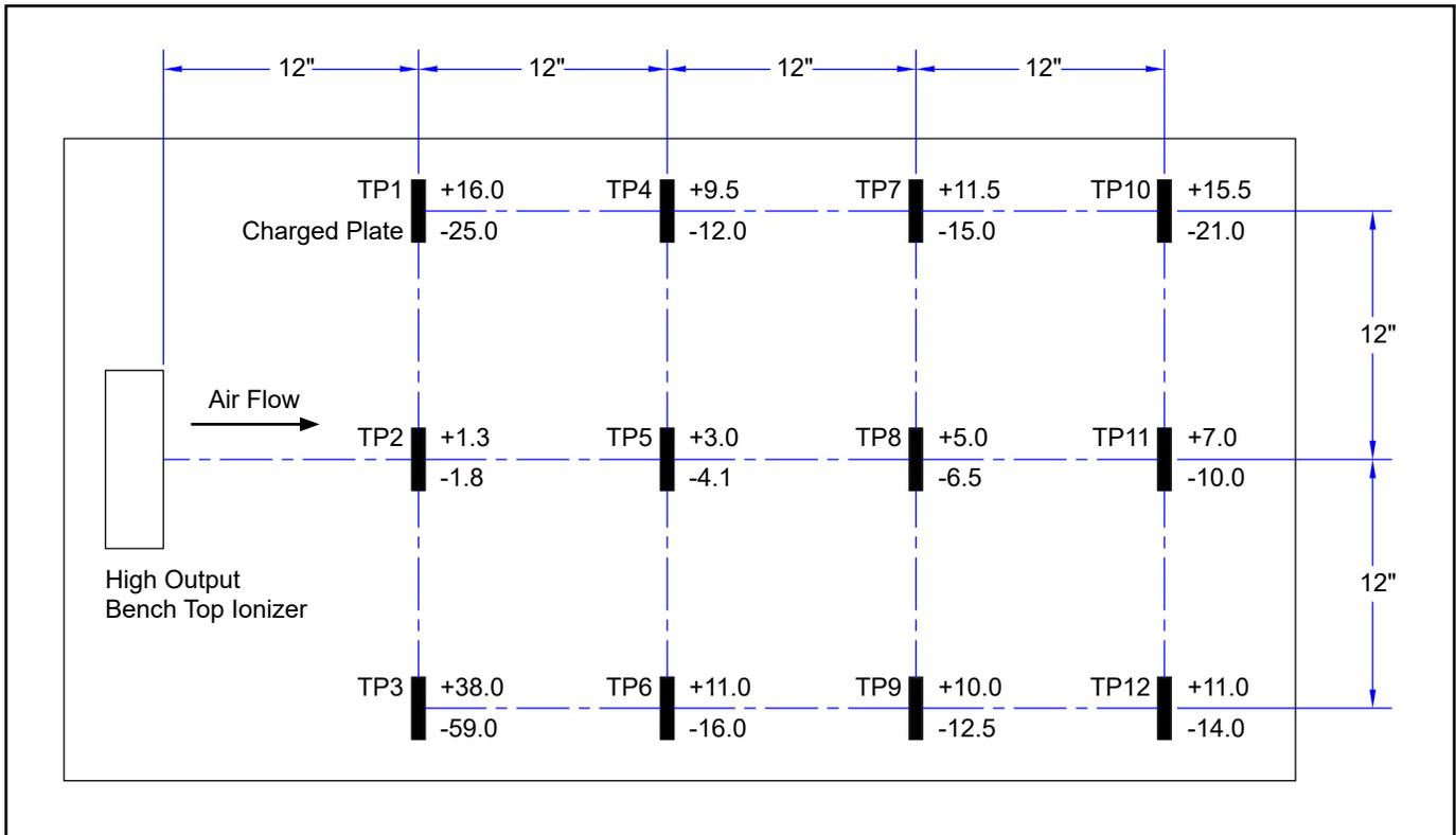
Figure 6. Neutralization (Discharge) Times at 100VAC, 50Hz input
